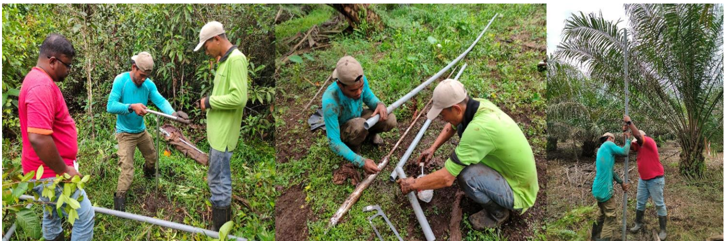
Figure 1. The pictures illustrating the piezometer installation process at BBEFR including the measurement of peat depth and installation of piezometers
